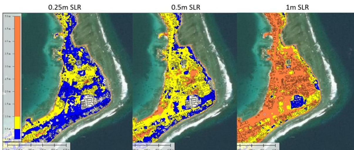
Figure 13: Example of 10 year ARI flood depth increments for part of D-U-D under 0.25, 0.5 and 1 m SLR scenarios
